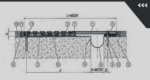
Setting for displacements till to +/- 300 mm
