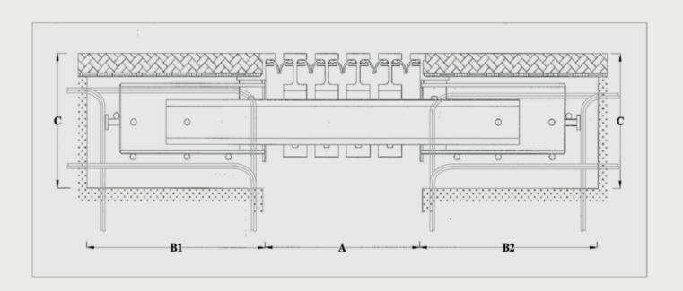
The laying of the joint, when allowed, must take place after a sufficient period of settlement of the flooring. The different settlement of the asphalt over time due to vehicular transit differs from the "joint" system where the use of high-strength mortars in the substrates and transition areas does not actually allow for any lowering.
